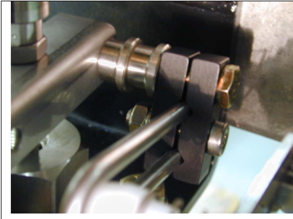
The first step is to check out the mechanical connections. Check that all parts of the assembly are tightly attached to the valve stem. Each type of valve will be slightly different. The important thing is that these cannot be easily moved. All connections must be tight.
