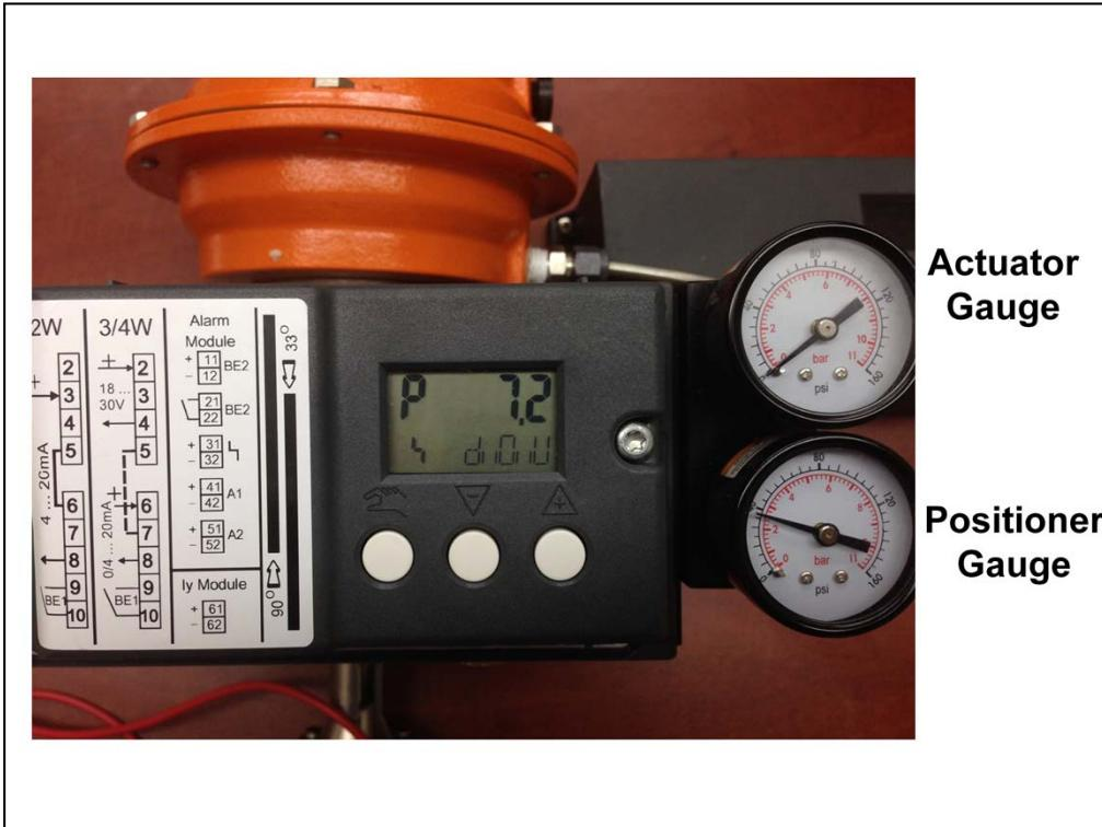
In Run 1, the positioner is trying to determine the direction the valve operates when given an input signal. If you get an error, it is simple to correct with the following steps...
