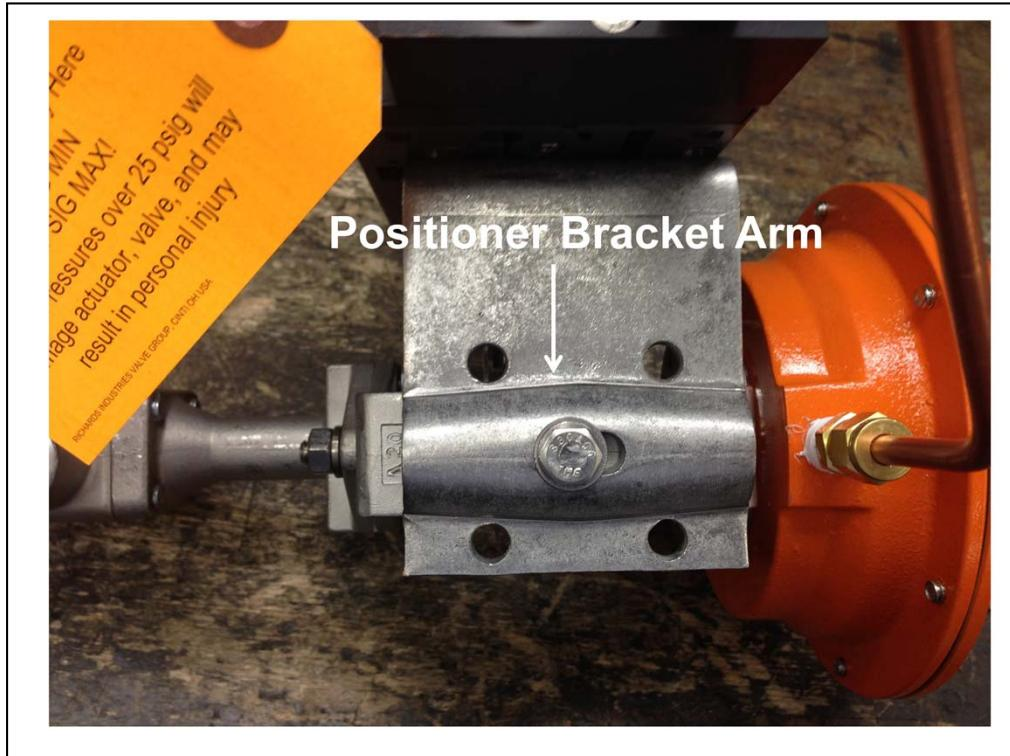
The last potential problem is that the Up band has been violated, meaning the positioner has entered an inactive zone. This indicates that either the transmission ratio selector or the pin on the positioner arm is not set properly. To correct...
