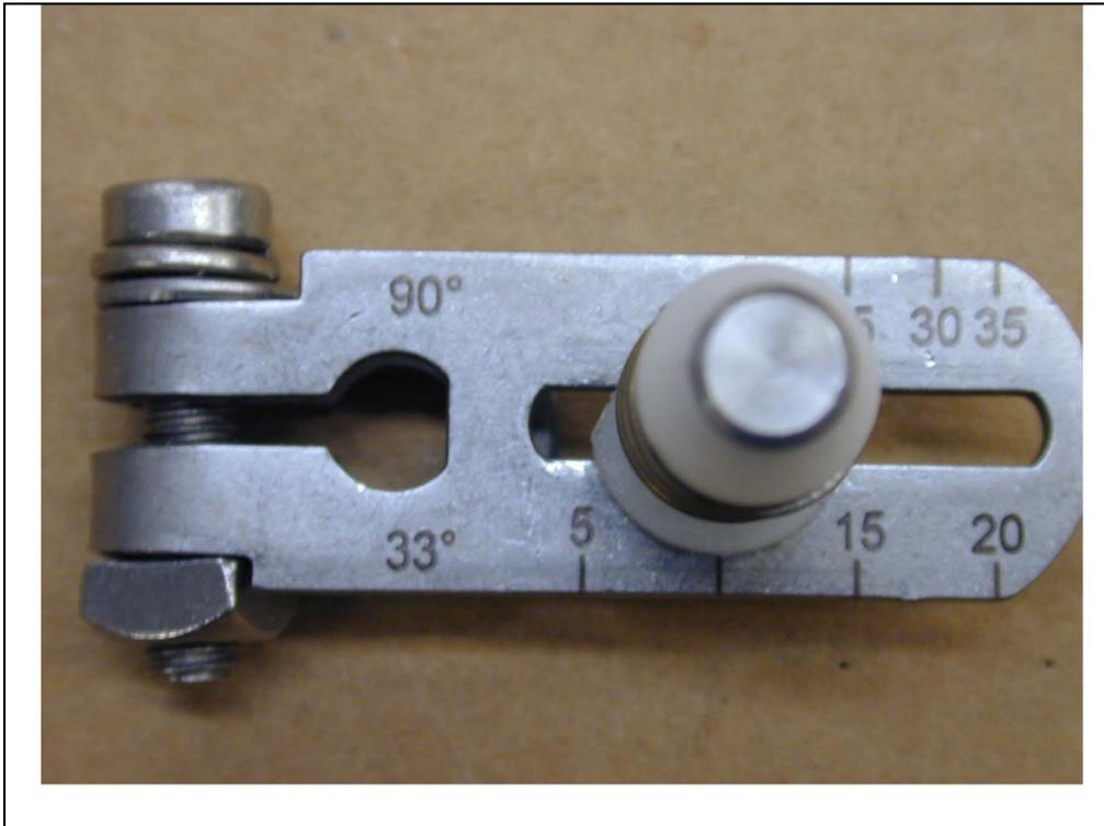
Verify that the pin is properly set on the positioner arm for the valve in question. You will need to know the stroke length of your valve in millimeters. There are separate scales for 33° and 90° setting, depending on the stroke of your valve.
