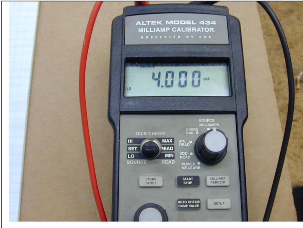
If everything checks out mechanically, move into testing the positioner. You will need the ability to change the input signal. This can be done through a control system or 4-20mA power source similar to one above.
