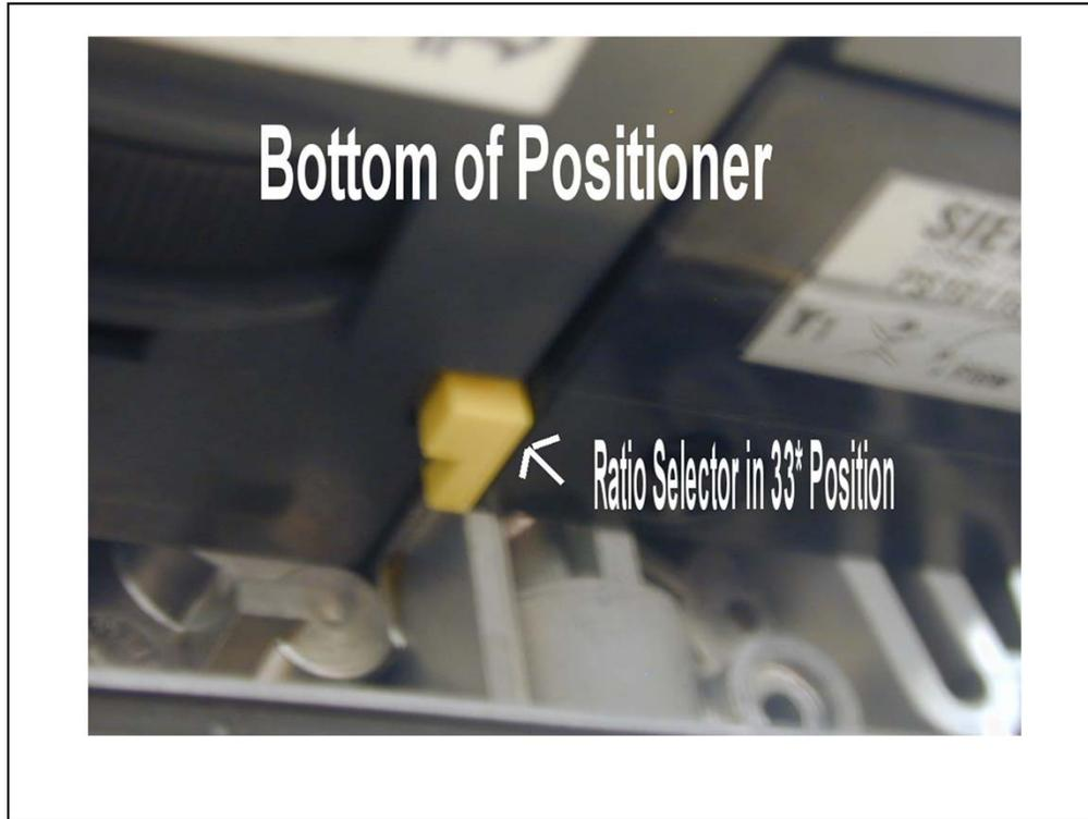
Make sure the transmission ratio selector is in the proper position. This is a yellow plastic bar that shifts vertically up and down inside of the positioner body.
