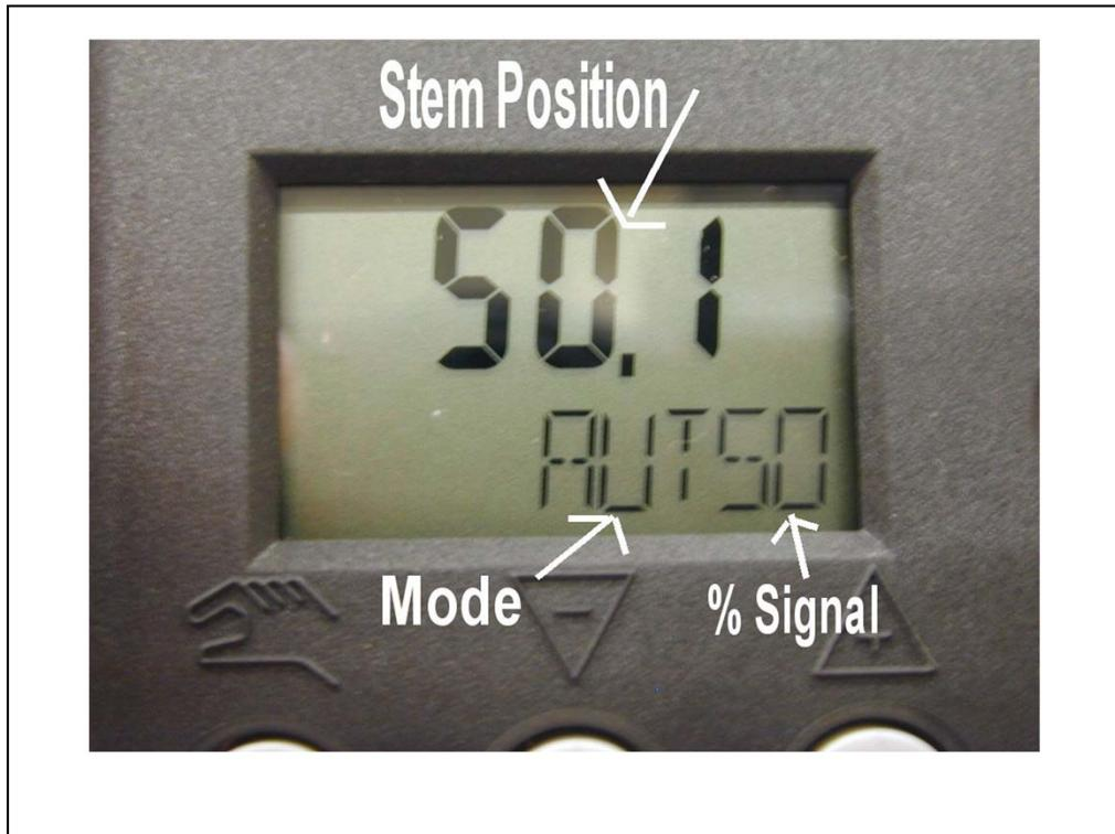
Double check that the valve is operating properly by changing the signal to the valve.
