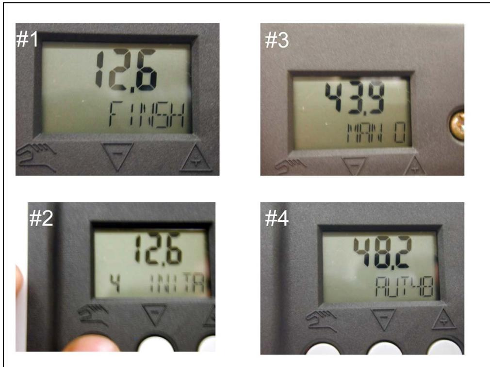
Step #1 - When the positioner is finished the display will read 'Finish'.
