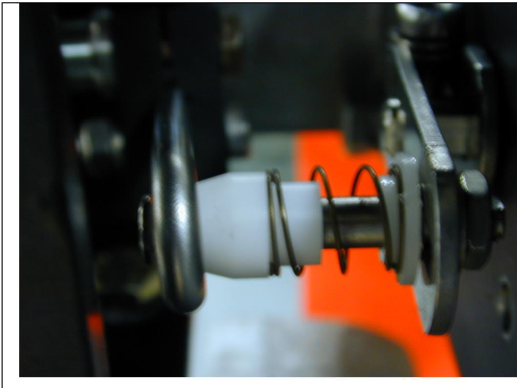
Now check to make sure the linkage is in connected and tight. The spring loaded nylon bushing on the positioner arm pin needs to be engaged in the mating arm. The bushing is spring loaded and must have spring tension holding the cone firmly in the bar.
